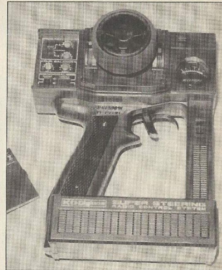
Space-gun like latest KO Digiace Tx design. Trigger operates speed, wheel the steering. Loose cover fits over adjustment panel. Harden Associates will be handling in G.B.
